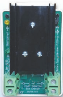
SC-2030 Solar Charger Located near batteries— connected to TM-2030 with telephone cable.
