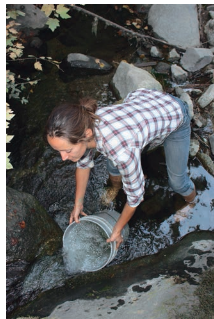
If you can get a container under the majority of the flow, the bucket method can be an easy way to measure it.
