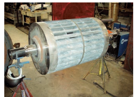
Above: Reaction runners come in various styles like this propeller type. Below: This impulse machine is a crossflow runner.
