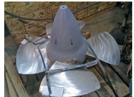
Above: Reaction runners come in various styles like this propeller type. Below: This impulse machine is a crossflow runner.
