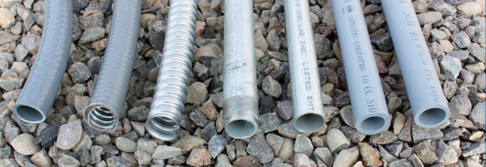
Three-quarter-inch conduit, left to right: Liquid-tight flexible nonmetallic conduit (LFNC), liquid-tight flexible metal conduit (LFMC); flexible metal conduit (FMC); rigid metal conduit (RMC); electrical metallic tubing (EMT); and polyvinyl chloride (PVC), schedule 80 and 40.
