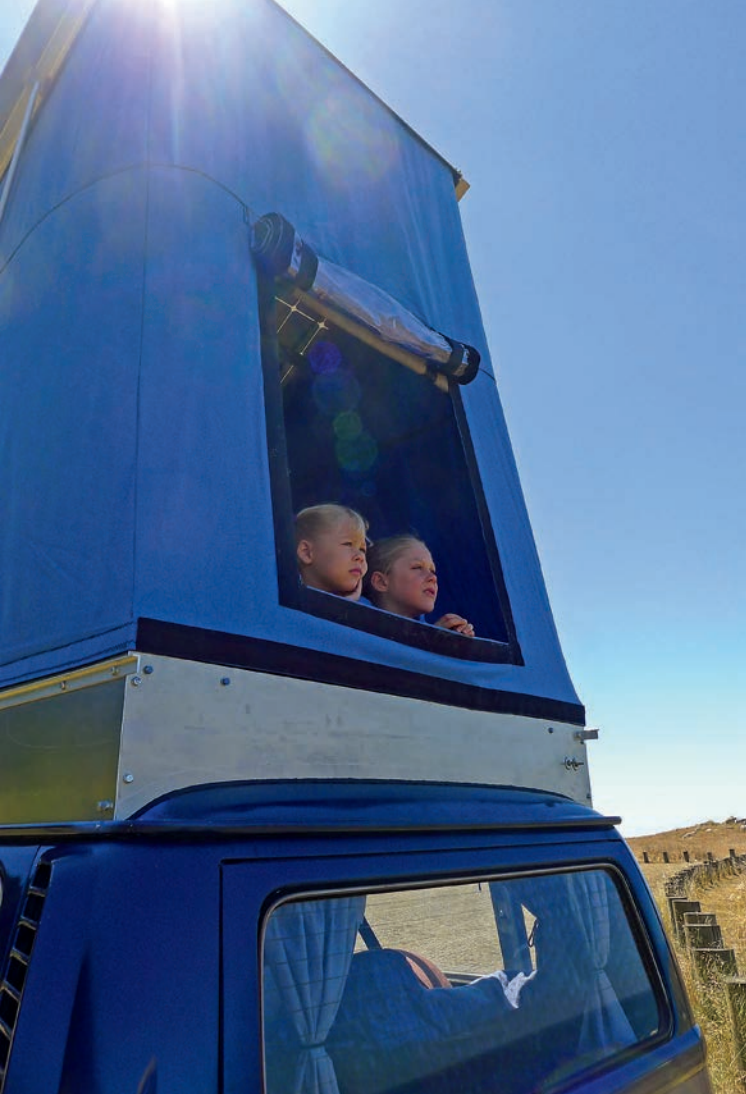
Left: The kids enjoy the view from the rooftop pop-up PV tent. The back sheets on the modules allow ambient light into the tent space.
