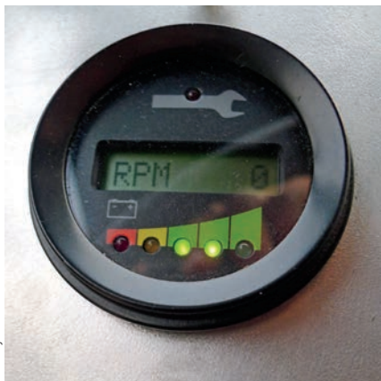
A Spyglass meter for the Curtis motor controller displays amps, volts, rpm, and controller and motor temperatures.
