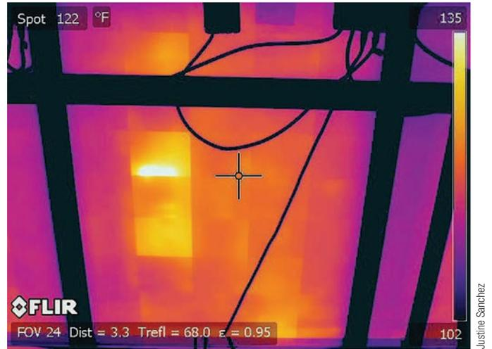
This thermal image, taken during system troubleshooting and testing, reveals hot intercell connections inside a PV module.
