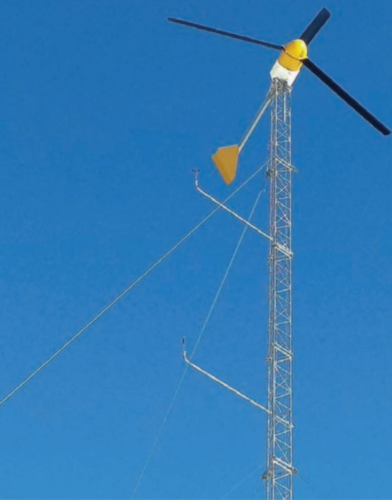
This Bergey Excel 10, installed in 2006, produces about 9 MWh of electricity each year.
