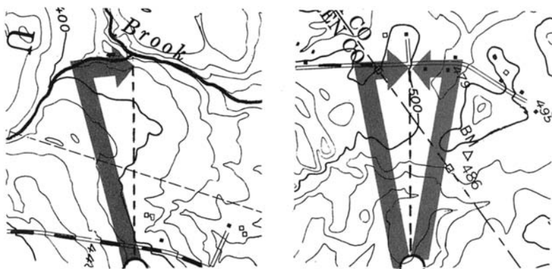
In aiming off toward a stream juncture, aim off upstream and follow the stream downstream to the juncture (left). Aim off left or right for a road juncture (right).
