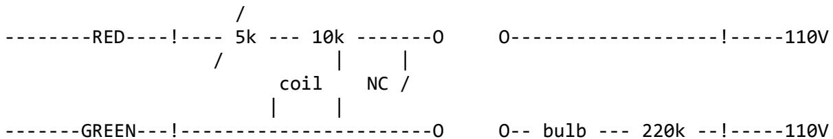
Make sure that the phone circuit (left) and the lamp circuit (right) are totally 100% separate, and in no danger of touching. Use wire nuts for all connections in 110V that are not to a terminal post, and tape them. For all wires that are exposed, use electrical tape or shrink-wrap tubing to insulate them. Glue the relay to the box or mount it on a stable PC board.
