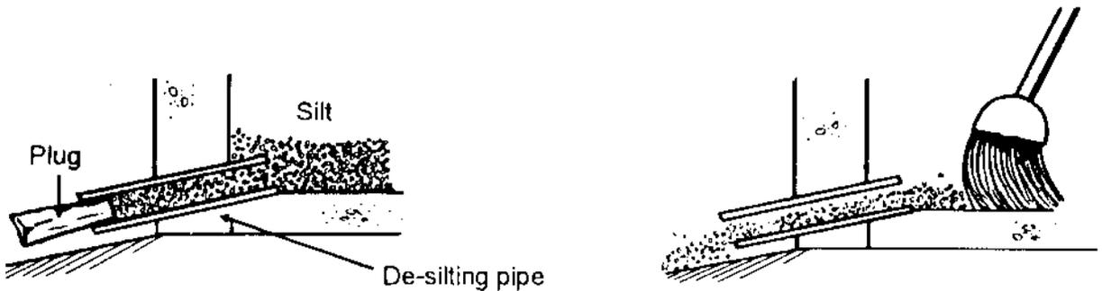
When a level overflow pipe is being used, a separate small diameter steel de-silting pipe should be set into the base of the tank and plugged. A shaped piece of wood can make a suitable plug. The plug is then removed to drain and de-silt the tank. Accumulated silt may need to be brushed towards the pipe to speed its removal.
