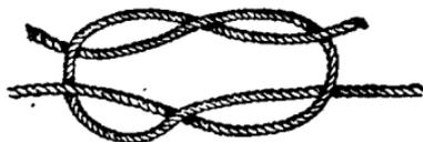
**False Reef or Granny.** If the ends are not crossed correctly when making the reef knot, the false reef or granny is the result. This knot is always bad.
