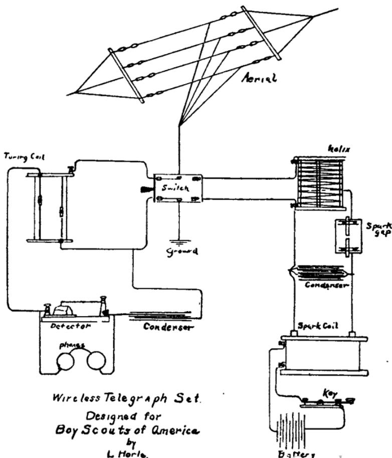
double-throw switch being used to switch from sending to receiving.
