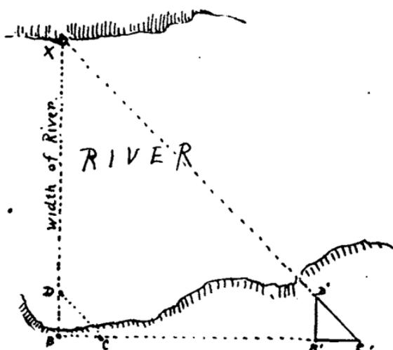
Another method is by the isosceles triangle. Make a right-angled triangle as above, with sides six, eight, and ten feet ( $A, B, C$ ); then, after firmly fixing the right angle, cut down the
