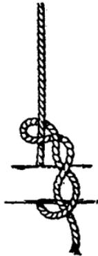
**Timber Hitch.** Used in hauling timber. Pass the end of the rope around the timber. Then lead it around its standing part and bring it back to make two or more turns on its own part. The strain will hold it securely
