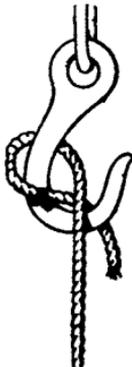
**Blackwall Hitch.** Used to secure a rope to a hook. The standing part when hauled tight holds the end firmly.
