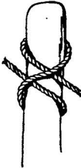
**Clove Hitch.** Used to fasten one pole to another in fitting up scaffolding; this knot holds snugly; is not liable to slip laterally.
