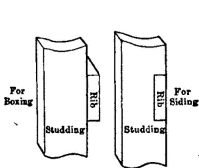
FIG. 76.—Attachment of ribs to studding.
