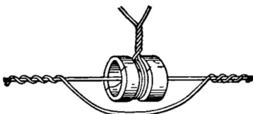
FIG. 39.—Swinging insulator.
