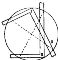
FIG. 122.—To obtain the center of a circle.
