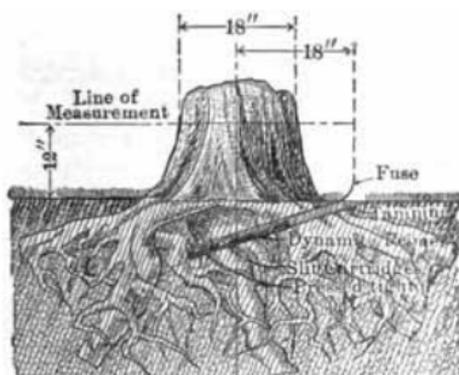
FIG. 69.—Charge placed too near surface.
