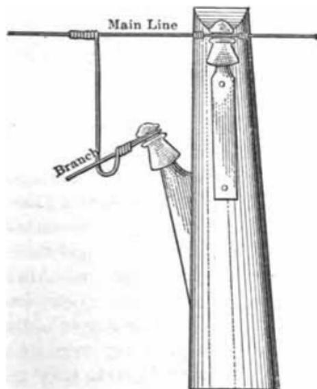
FIG. 43.—Branch-line connection.
