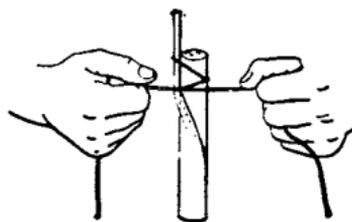
FIG. 62.—Tying the fuse into the cartridge.
