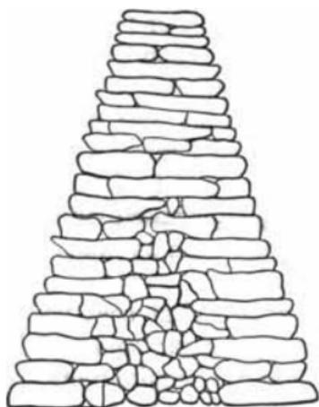
FIG. 87.—Cross-section of a stone fence.
