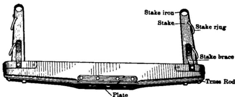
FIG. 145.—Front or "rocking" bolster.
