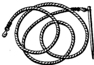
FIG. 23.—Picket pin and rope.
