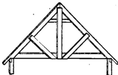
FIG. 82.—Self-supporting roof.
