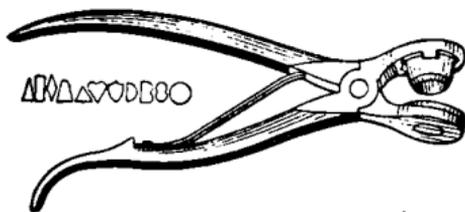
FIG. 218.—Ear punch and dies.
