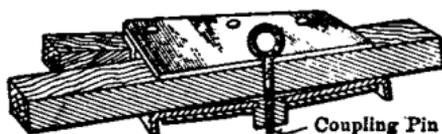
FIG. 142.—Sectional view of reach plate.
