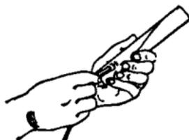
FIG. 60.—Inserting cap in cartridge.
