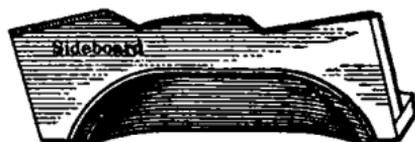
FIG. 154.—Rub iron. "Cut-under" type.
