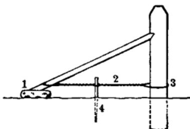
FIG. 97.—Brace for corner post.
