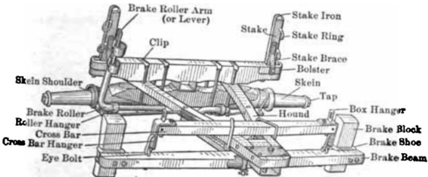
FIG. 146.—Rear gear with mountain brake.
