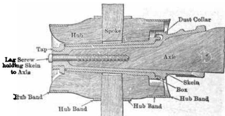
Method of attaching skein to wood axle.
