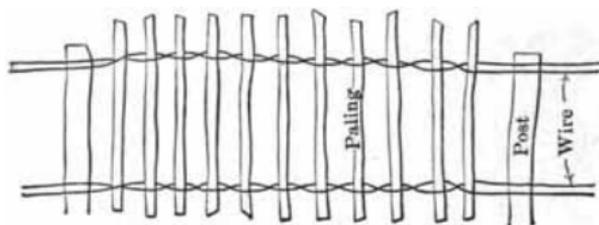
FIG. 93.—Picket or "paling" fence.
