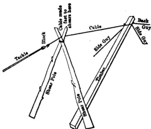
FIG. 127.—Erection of timber with shears.
