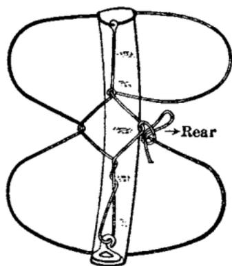
FIG. 131.—Top view of diamond hitch.
