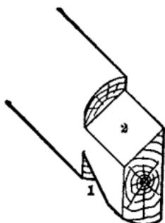
FIG. 85.—Notches for wall logs.
