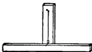
FIG. 126.—Substitute for level-plumb.
