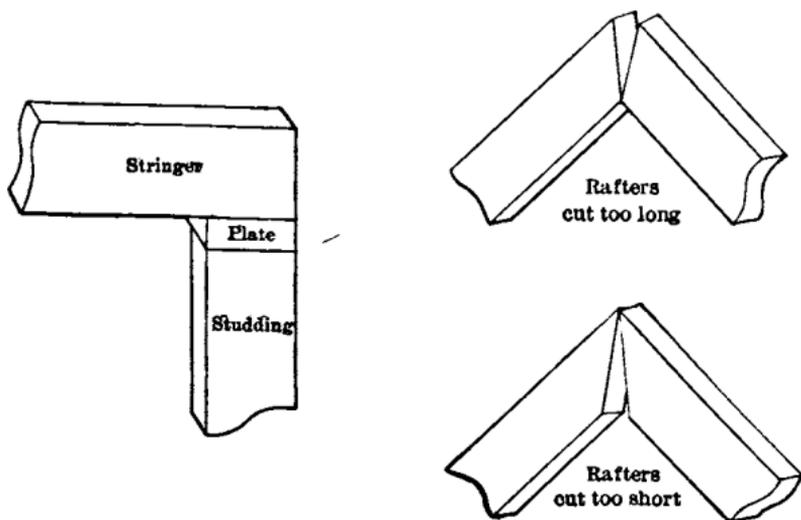
FIG. 79.—Attachment of stringer to plate
