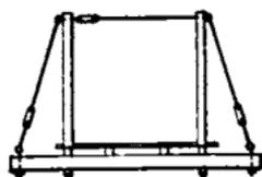
FIG. 55.—Method of guying bridge "rafters."
