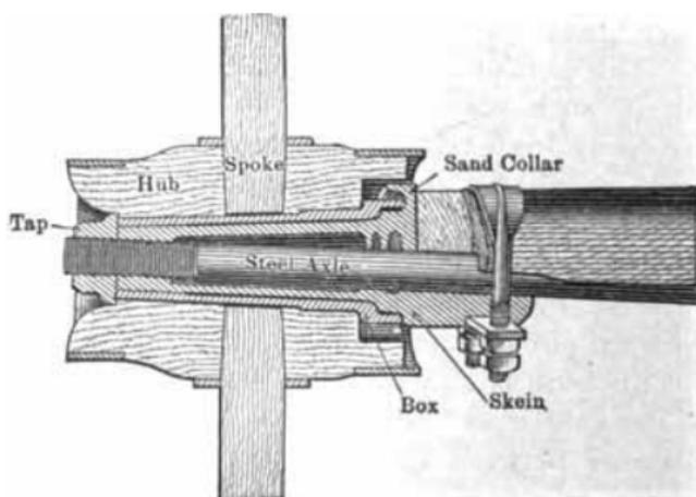
Method of attaching skein to steel axle.
