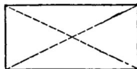
FIG. 123.—To obtain the center of a rectangle.
