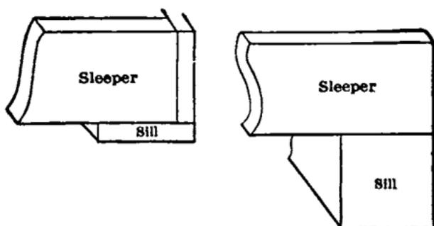
FIG. 73.—Attachment of sleepers.
