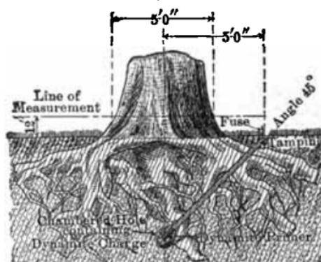
FIG. 71.—"Chambered" or "sprung" bore-hole.
