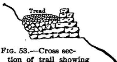
FIG. 53.—Cross section of trail showing construction of retaining walls.
