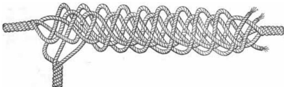
Incorrect method of starting an eye splice.
