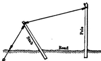
FIG. 33.—Stub for telephone pole.
