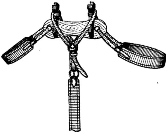
FIG. 19.—Full-rigged pack-saddle. (Single rig.)
