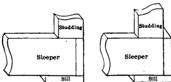
FIG. 75.—Attachment of corner studding.
