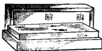
FIG. 112.—Oilstone mounted in block.
