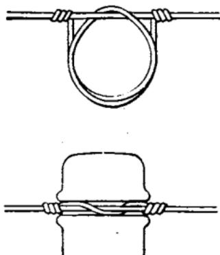
FIG. 36.—Figure 8 tie for iron wire.
