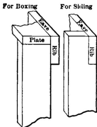
FIG. 77.—Attachment of plates.
