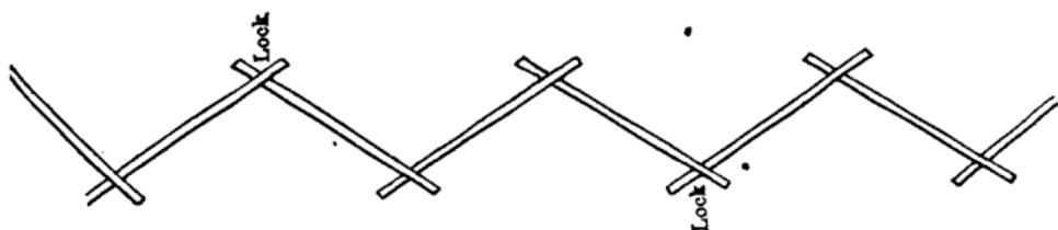
FIG. 89.—Worm rail fence. Method of laying ground rails.
