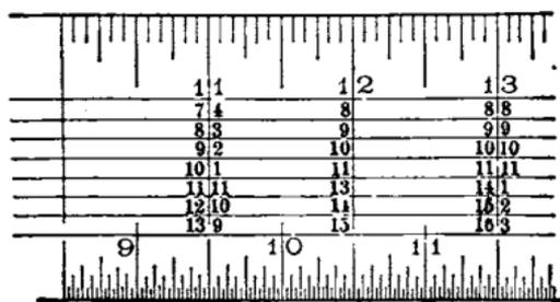
FIG. 114.—Board Scale.
