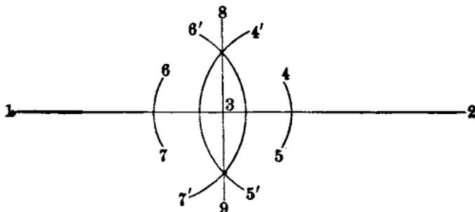
FIG. 124.—To erect a perpendicular without a square.
