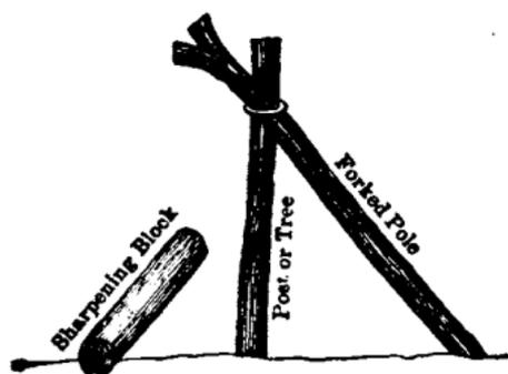
FIG. 98.—Rack for sharpening posts.
