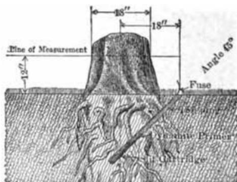
FIG. 66.—Correct location of charge in tap root.
