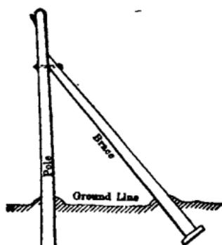
FIG. 31.—Brace for telephone pole.
