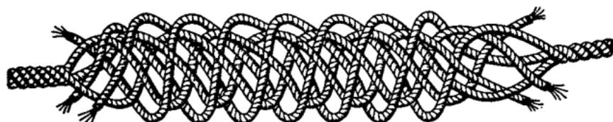
FIG. 229.—Permanent eye splice.
