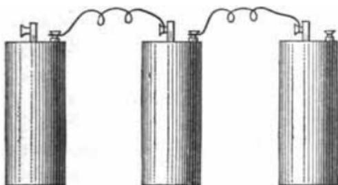
FIG. 46.—Connection of batteries.
