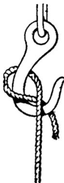
**Blackwall Hitch.** Used to secure a rope to a hook. The standing part when hauled tight holds the end firmly.
