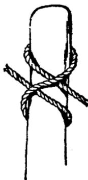
**Clove Hitch.** Used to fasten one pole to another in fitting up scaffolding; this knot holds snugly; is not liable to slip laterally.
