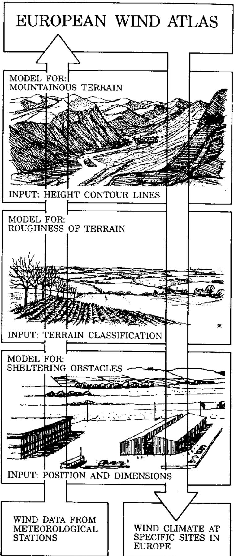
Meteorological models were used to calculate the regional wind climatologies from the raw data. In the reverse process - the application of the Wind Atlas - the wind climate at any specific site may be calculated from the regional climatology.
