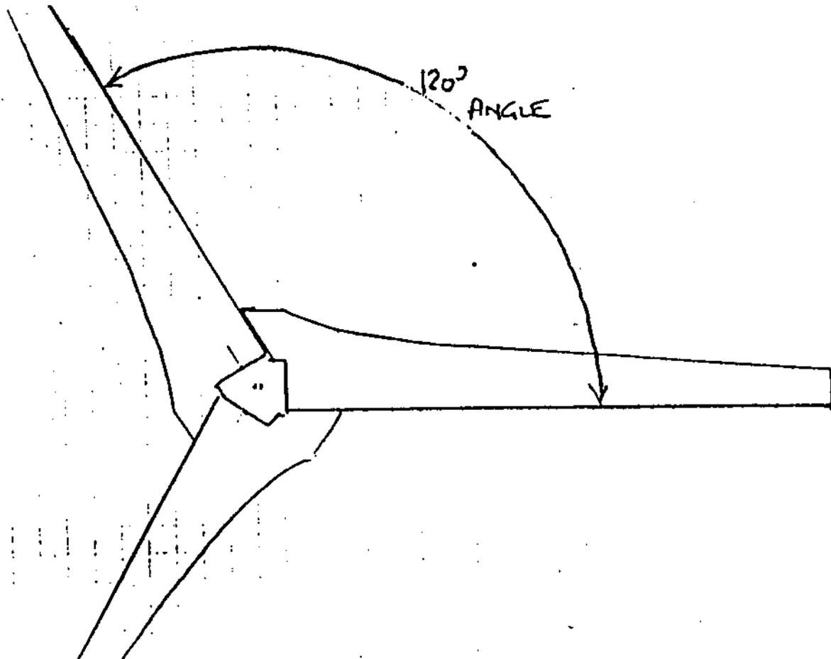
When you have the blades all fitting snugly as described, cut two hexagons out of sturdy plywood (minimum 9mm better 12mm) as shown in figure 12:
