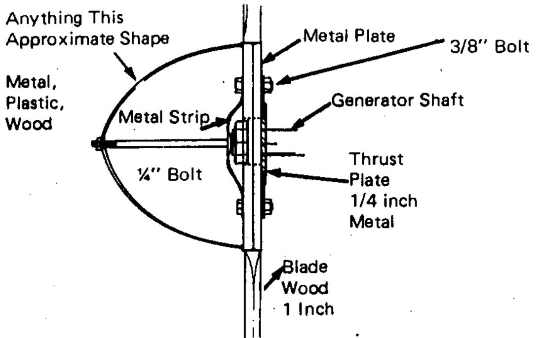
**Fig. 1 HUB ASSEMBLY (Detail)**
