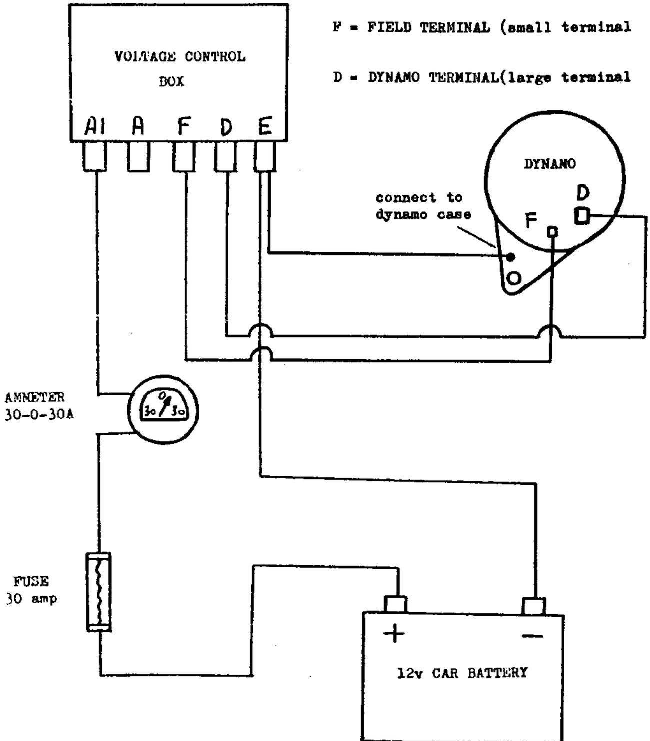
FIG. 7 - GENERATOR WIRING DIAGRAM
