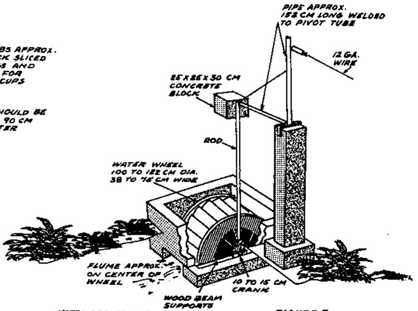
NOTE: CRANK CAN BE ADDED TO OTHER END OF SHAFT AT 90° ANGLE TO FIRST CRANK TO ATTACH MORE POWER TRANSMITTING WIRES
