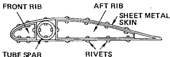
The usual material for this design is aluminum, but you will have to be careful in planning this type of blade to get the skin to take both the curvature of the airfoil, and blade twist. Try constructing a test blade with paper. Rivets and epoxy bonding will attach the skin, ribs, and spar together. Rivets may be aircraft aluminum, or steel "pop-rivets".
