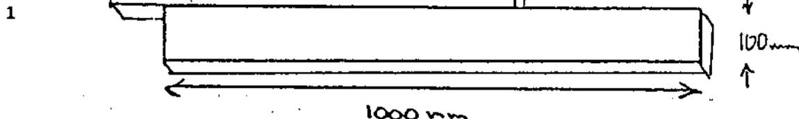
If you do not have enough wood, you may be able to work out a way of producing the final shape by cutting what you have into triangles. Use the same epoxy as for the alternator job. Other glues may be ok, but epoxy is definitely very suitable. Clamp the pieces together very firmly while the glue sets.
