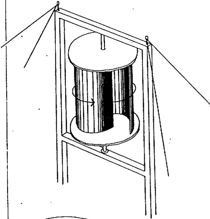
Fig 7. Savonius rotor.
