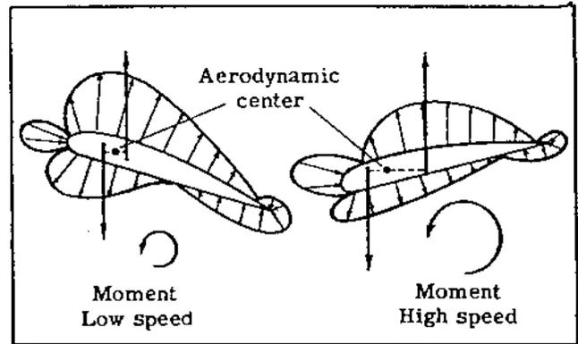
Fig. 3-5. The moments created by the unsymmetrical airfoil at two different airspeeds. The angles of attack and pressure patterns around the airfoil have been exaggerated.
