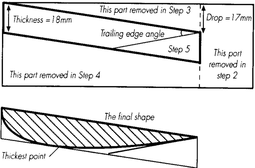
back (not the windward face) until you have a sharp edge, less than a millimetre wide, bevelled at the  $20^\circ$  angle shown. Set the work up with light shining onto the trailing edge, so you can easily see how wide it is. The finished edge should be under 1 mm wide.
