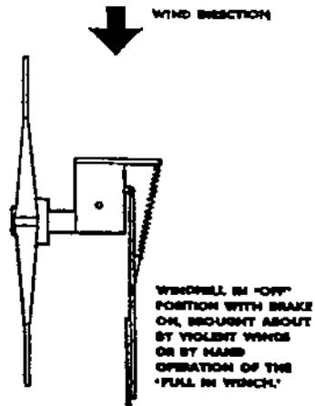
The Hercules windmill is designed to work in low windspeeds, as the windspeed increases the automatic governing device comes into action and operates as follows—
