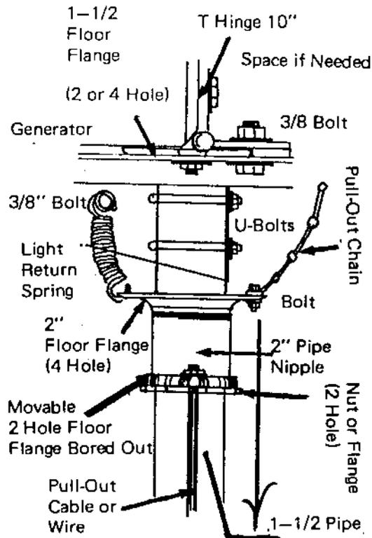
**Fig. 6 MANUAL PULL-OUT ASSEMBLY (Side View)**
