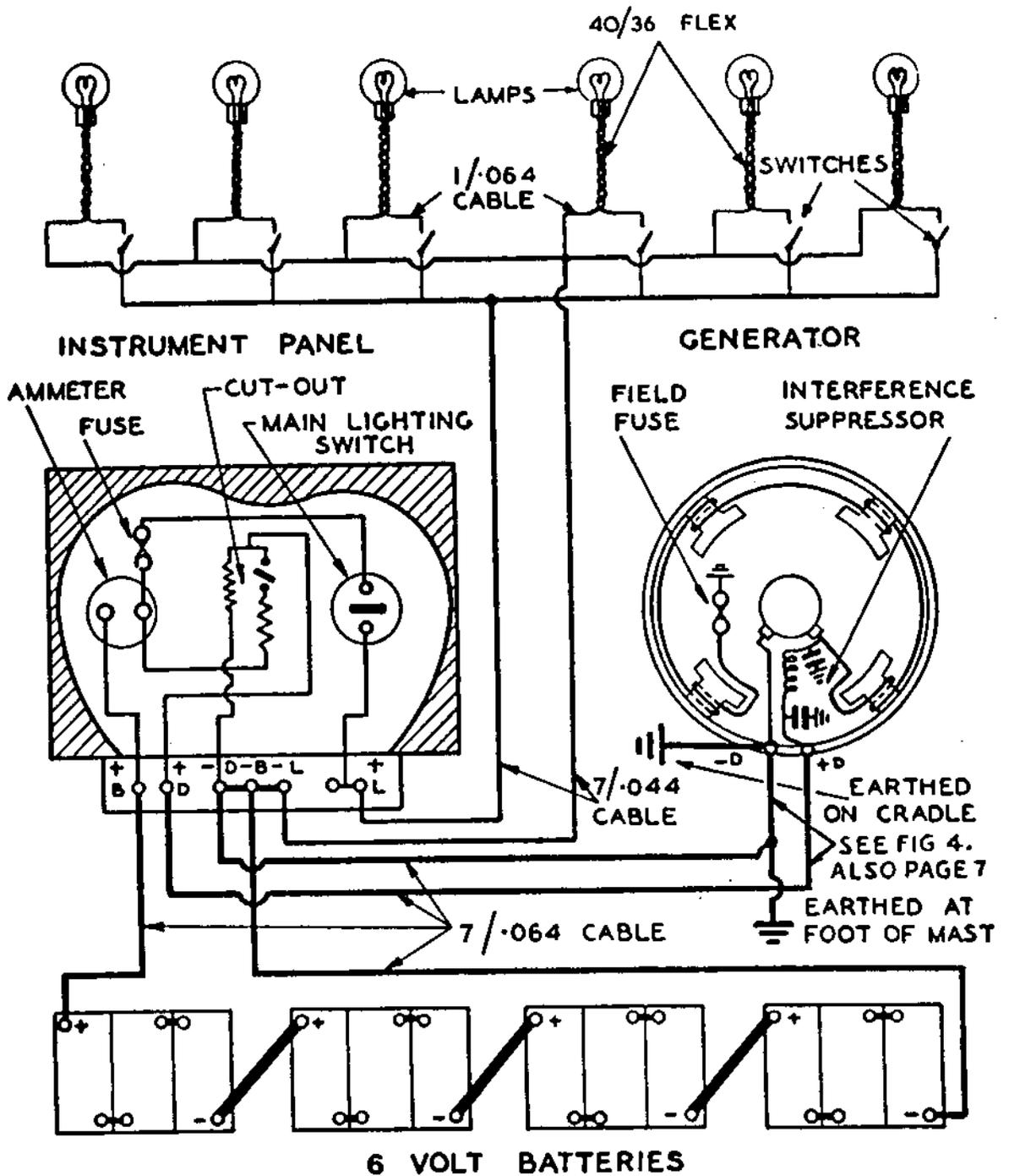
FIG. 86. Wiring diagram for Lucas "Freelite" machine
