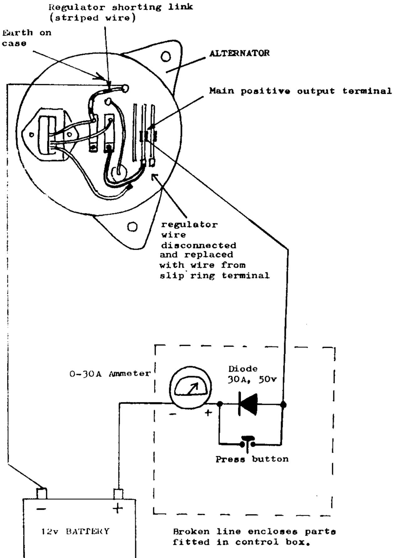
**FIG. 6 - GENERATOR WIRING DIAGRAM**
