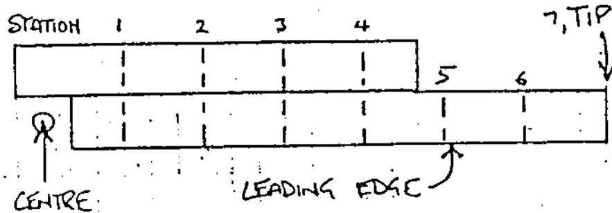
Next you need to produce the correct taper : ie get the blade "chord width" right at each station. In all that follows, the leading edge remains untouched, as a sort of reference line. Measure the width from the leading edge at each station, join the dots with a line, and cut away the surplus wood, as shown in fig 3:
