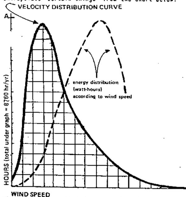
The chart is called the velocity distribution curve. It is a similar shape for all wind power locations, and gives a good indication of the amount of time the wind blows at a particular wind speed.
