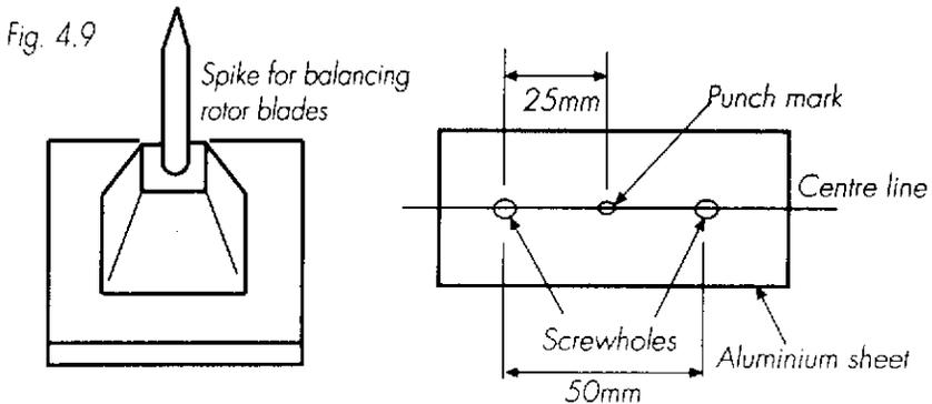
nail or similar, driven into a wooden support, and sharpened with a grinder. The spike engages with a punch mark at the exact centre of the rotor.
