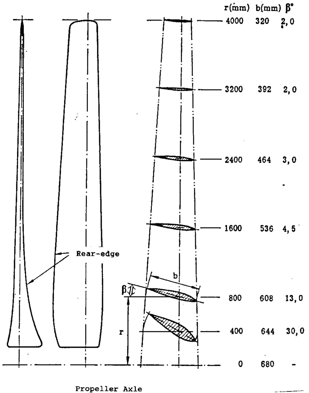
Figure 3. Propeller blade for a 3-blade propeller
