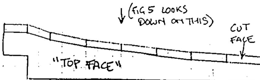
Now we need to draw a line to mark the position of the trailing edge of the blade on the newly cut face. At each station, measure the prescribed amount (figure 5) from the "top face" along the newly drawn lines on the cut face. Mark a dot on each line at the correct distance from the top face. Join the dots, to produce the trailing edge line of the blade, as shown in figure 5. The thickness of the wood is exaggerated to make it easier to see what is happening:
