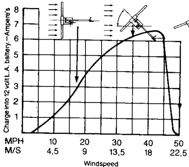
Above: The Furlmatic's output current versus windspeed curve.
