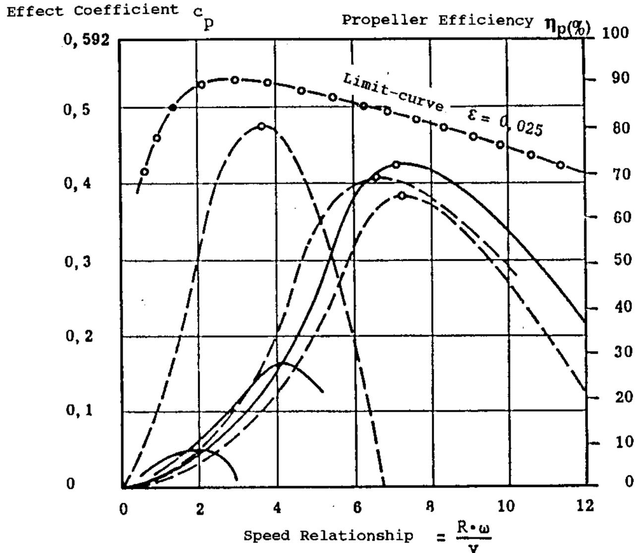
Figure 4. Effect coefficient for different propeller types
