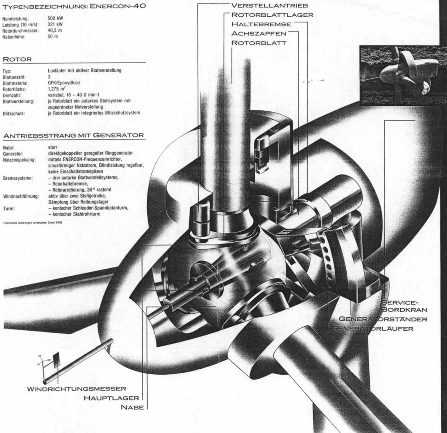
**Enercon 500 kW Wind-turbine without gearbox,
