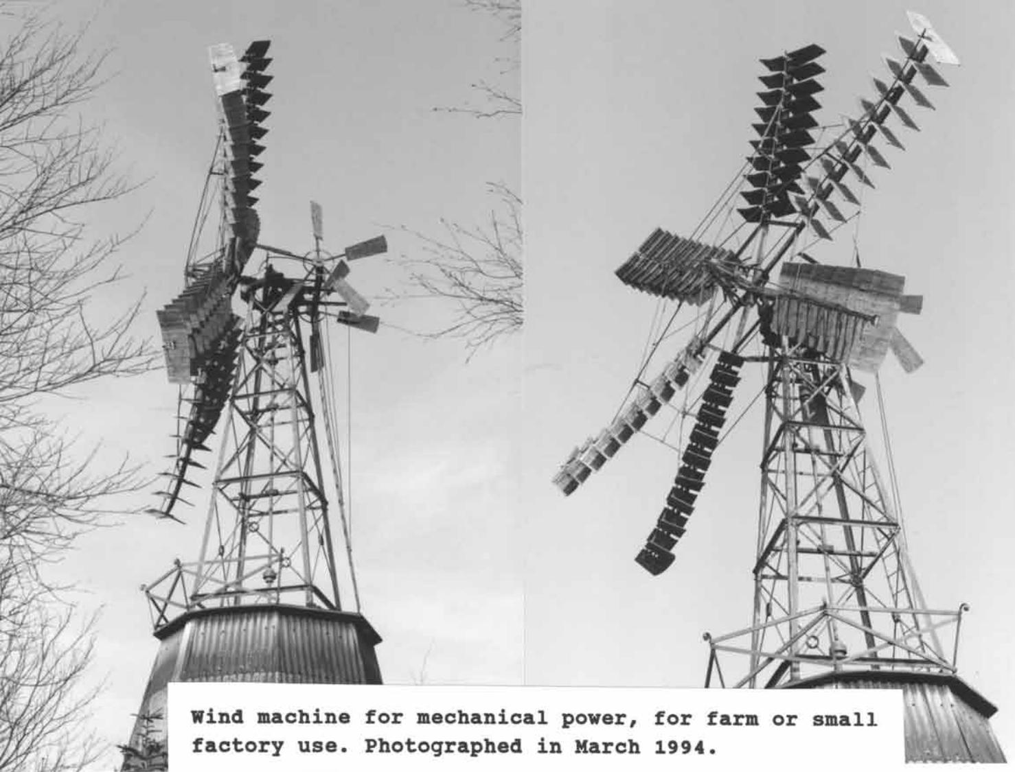
Wind machine for mechanical power, for farm or small factory use. Photographed in March 1994.
