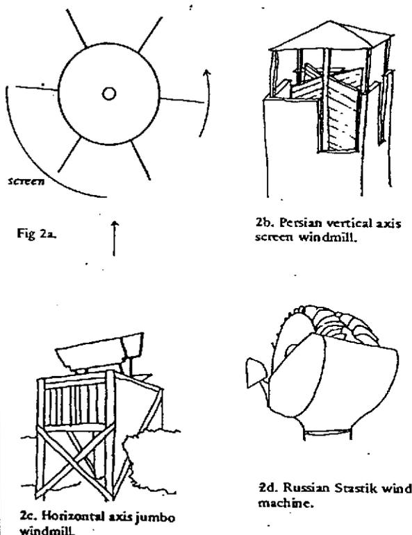
'merry-go-round' windmills; see Fig 2b), or a horizontal axis (these are sometimes known as 'jumbo' windmills; see Fig 2c). The Russian Stastik windmill (Fig 2d), in which the whole machine was kept oriented into the wind was a horizontal-axis version.
