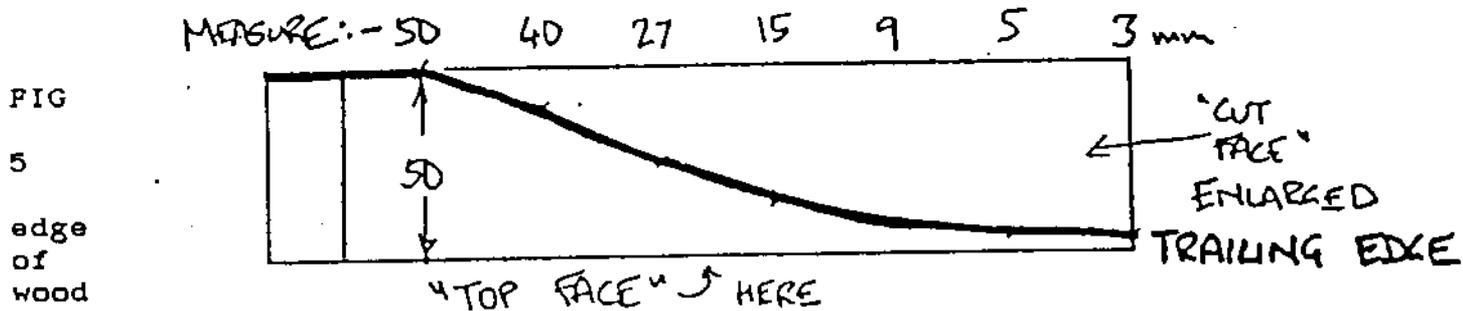
The trailing edge line is shown in bold in figure 5. This line is all that will remain of this face of the wood when you have finished the job. Now it is time to tackle the windward face (front) of the propeller blade. For simplicity, I recommend a flat front face, although some people cut them concave. When I say flat, I mean that the line between leading and trailing edges is straight. The face itself is not flat, but twisted, due to the strange curve of the trailing edge.
