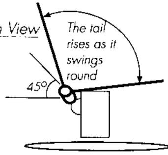
Seen from above, the axis of the tail hinge should make an angle of 45 degrees to the rotor plane.
