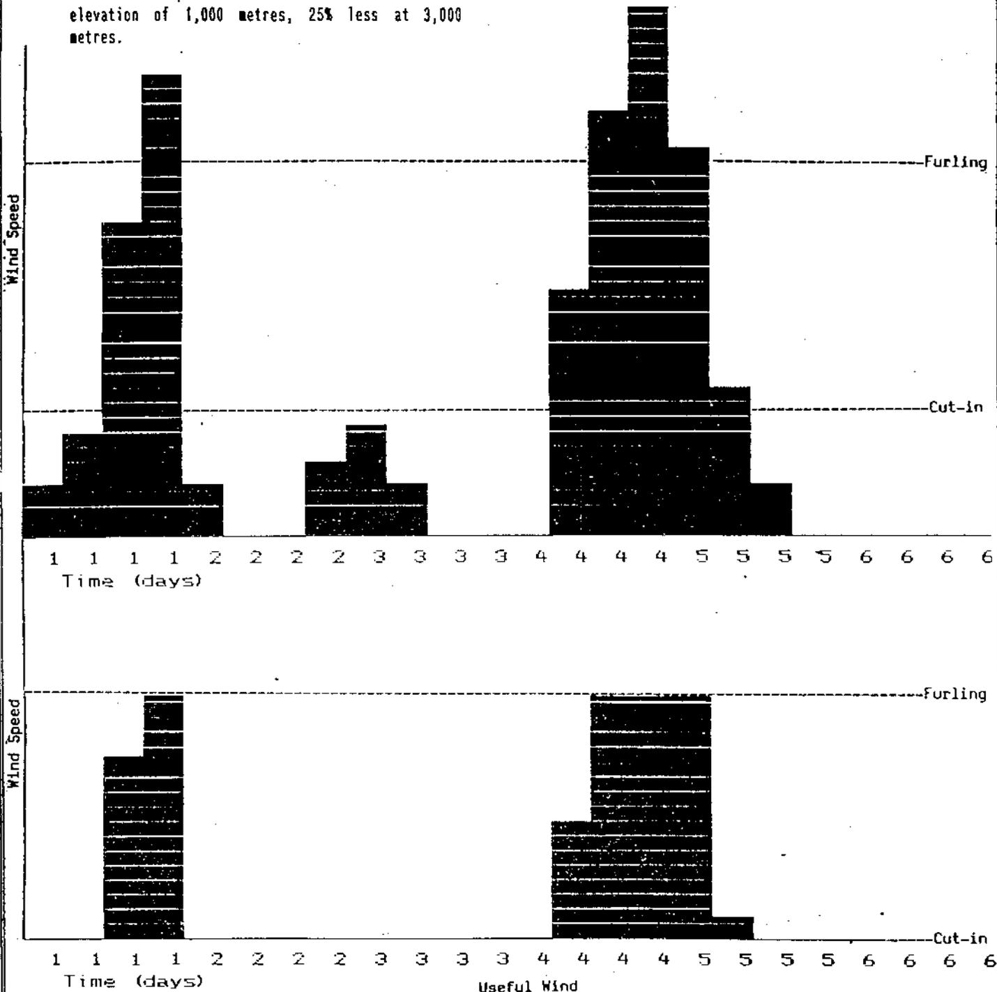
The period over which there is no wind with sufficient force to generate power is the period when either the battery storage or another energy source must provide the required power.
