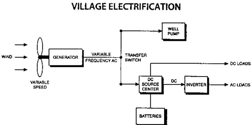
*Figure 11-8. One scheme for using small wind turbines to serve a variety of loads in a village electrification program.*
