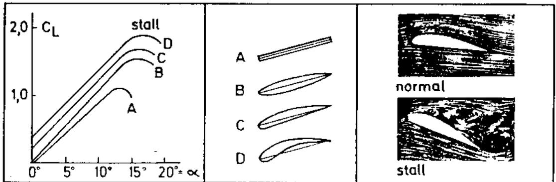
Figure 9. Angles of attack, and Lift-coefficients profile forms.
