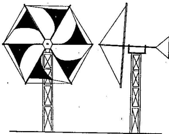
to utilize low wind speeds down to about 2.5 m/s (6 mph), and their ability to start under load, high solidity machines are generally used for mechanical purposes—such as pumping and corn grinding.
