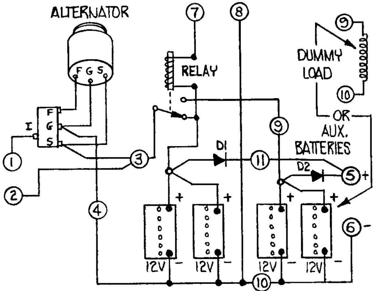
NOTE: IN THIS DRAWING, D1 & D2 PERMIT SIMULTANEOUS USE OF MAIN & AUX. BATTERIES. THIS OUTPUT CAN BE WIRED AS SHOWN IN FIG. 4-8, WHICH IN TURN CAN BE WIRED AS SHOWN IN THIS DRAWING (USING DIODES).
