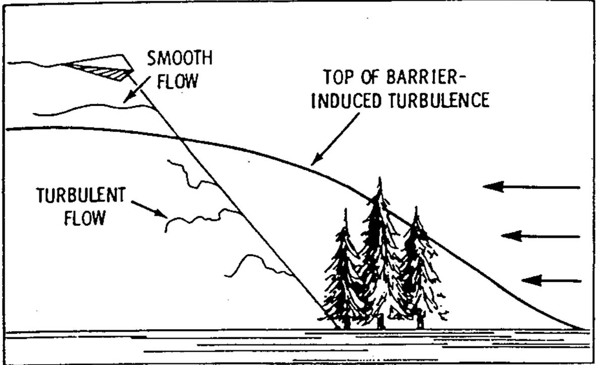
Wind turbulence can be visualized by studying a small river with many disturbances such as boulders. The wind follows the same flow pattern.
