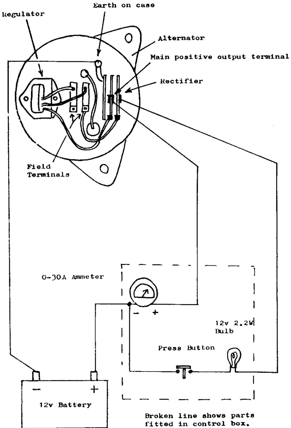
**FIG. 5 -- 12 VOLT UN-REGULATED VERSION WIRING DIAGRAM**
