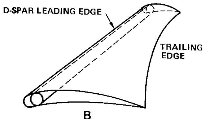
These blades are easily made with a tube spar, a stretched cable trailing edge, and a plasticized fabric (the fabric pores are sealed against air leakage) membrane. The membrane changes curvature in response to changing airflow, and thus generates high lift quite efficiently. The membrane must be stretched fairly tight for best performance. An ideal membrane can be made from the light weight nylon fabric that backpacking tents are made with, or extra light sail cloth, as used on hang gliders.
