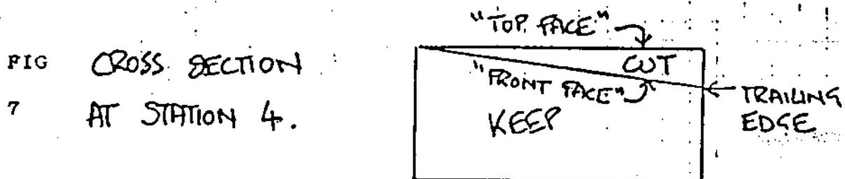
Having cut the front face, the next step is to make the blade the correct THICKNESS. Near the root, the thickness should be about 15% of the chord width. It drop to about 12% of the chord width at the tip. The actual thicknesses I recommend are shown in figure 8.
