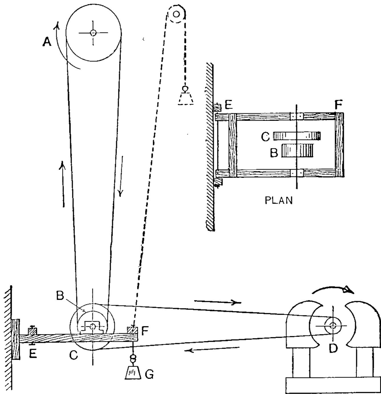
FIG. 75.—Driving Belt Arrangement for Wind Electrical Plant.
