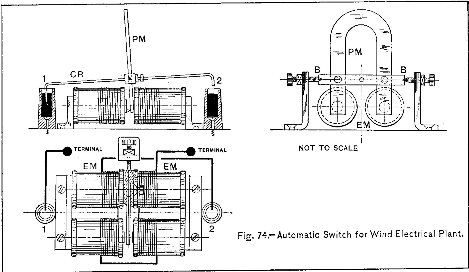
Fig. 74.— Automatic Switch for Wind Electrical Plant.
