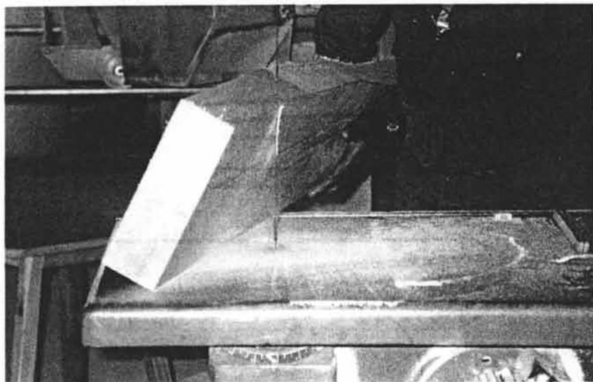
necessary to use callipers (Fig. 4.4) to check the actual thickness at each station. Measure how many more millimetres need to be removed, write it in pencil on the workpiece at each station, and resume shaving the piece down until the thickness is correct to within 0.5 mm.
