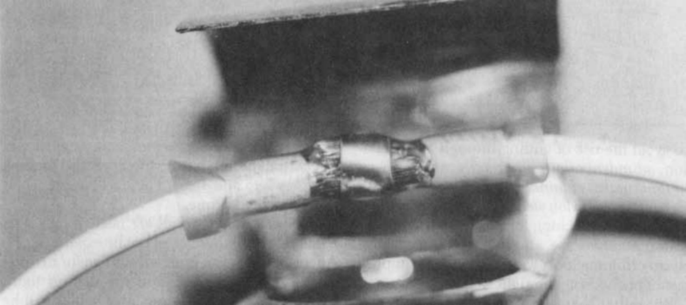
**Figure 3-47. Low-temperature solder connection with built-in heat shrink tubing. The solder sleeve is just beginning to melt into the lay of the two cables. At the same time the heat shrink sleeve is starting to clamp down around the cables.**
