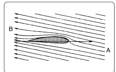
*Air flow around an aerodynamic profile*
