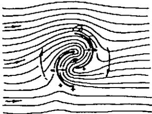
Air streaming and pressure differences around a Savonius rotor (From *Mechanical Engineering*, May 1931 p.334).
