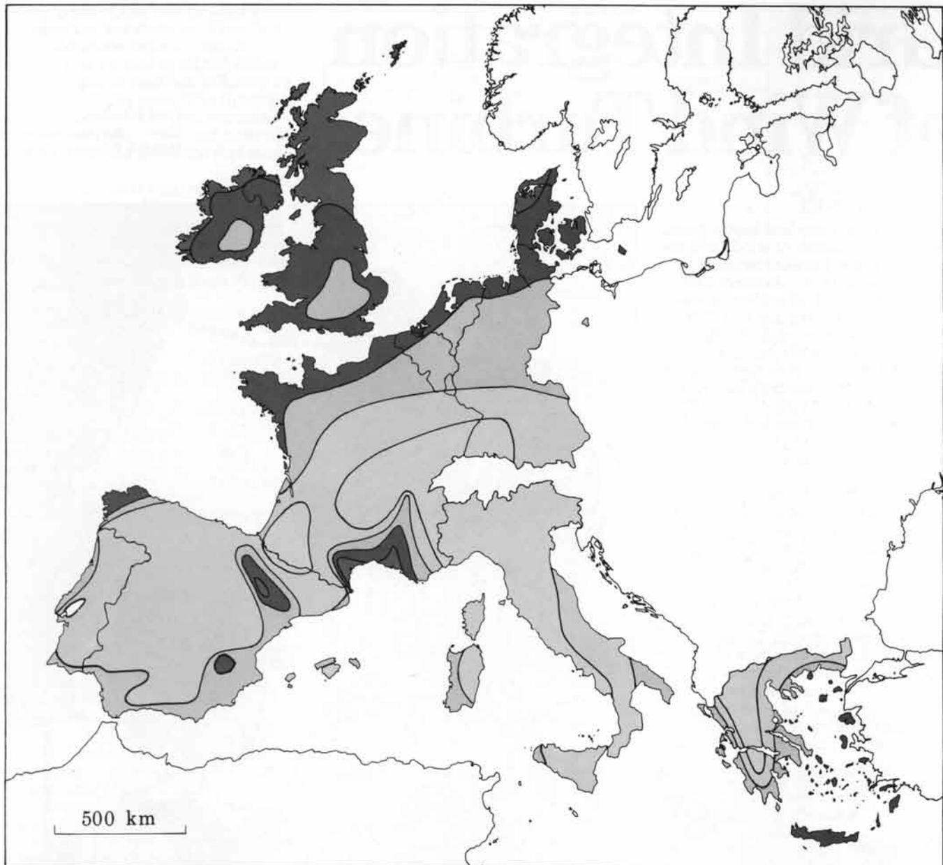
Wind resources<sup>1</sup> at 50 metres above ground level for five different topographic conditions
