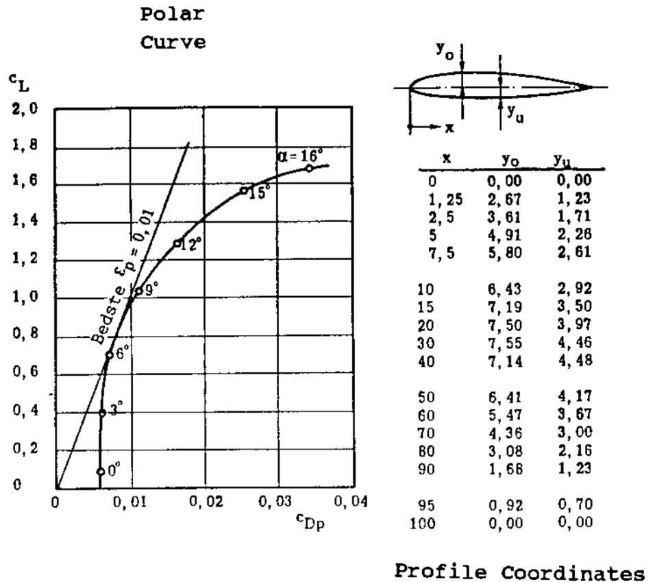
Figure 2. NACA 23012 Wing Profile
