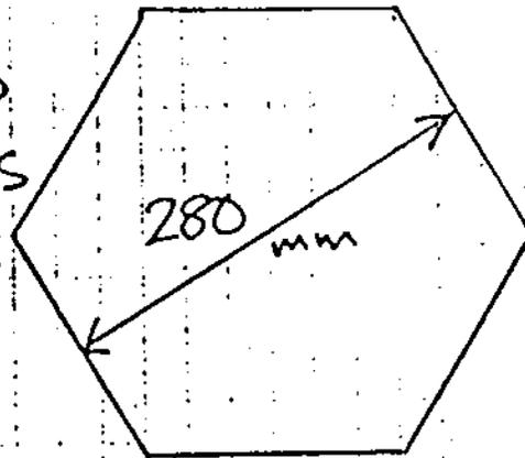
Sandwich the centre of the propeller between these two hexagons and fasten the whole together with a pattern of 2" woodscrews. I used 36 screws in all. Obviously you need to position the blades carefully before you start driving in screws.
