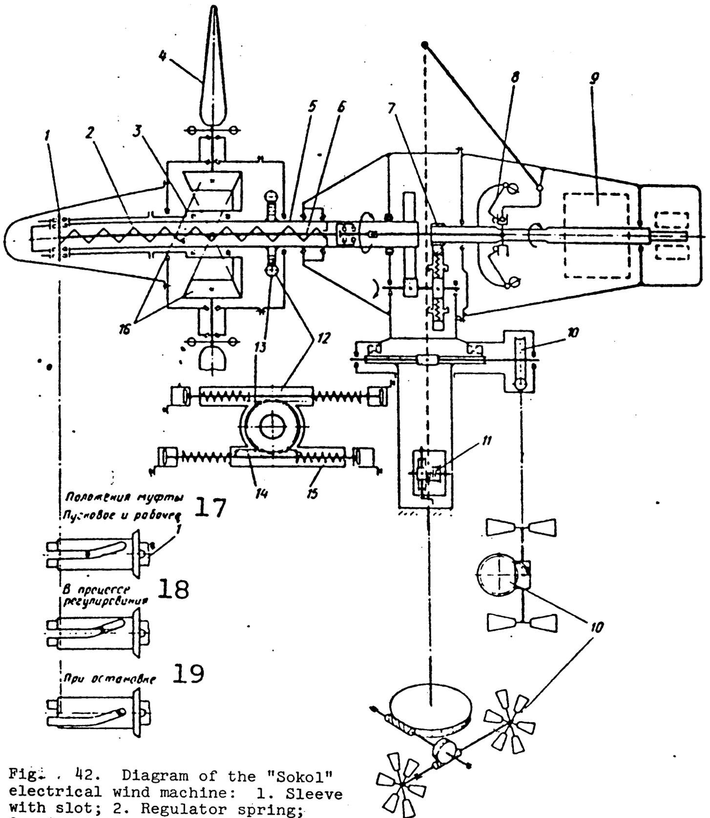
Fig. 42. Diagram of the "Sokol" electrical wind machine: 1. Sleeve with slot; 2. Regulator spring; 3. Kinematic connection gear; 4. Windmill; 5. Main shaft; 6. Regulator rod; 7. Reduction gear; 8. Centrifugal regulator; 9. Generator; 10. Orientation mechanism; 11. Starting-stopping windlass; 12. Moment regulator; 13. Toothed wheel; 14. Toothed racks; 15. Moment regulator spring; 16. Stroke spring; 17. Starting and working positions of sleeve; 18. In the process of regulation; 19. When stopping.
