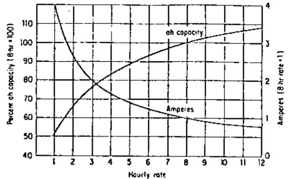
FIG. 5. CAPACITY-RATE CURVE BASED ON 8-HR. RATE
