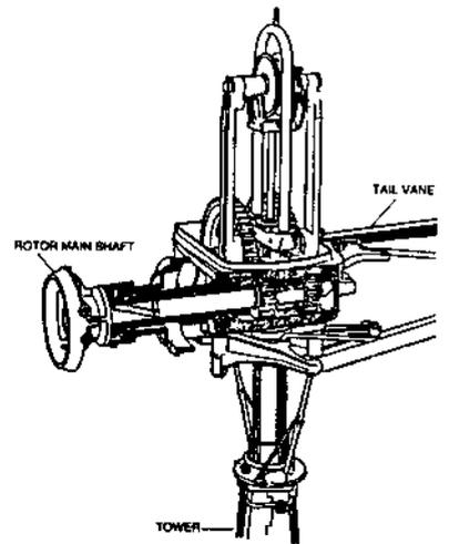
Most farm windmills are back-gearred, that is, the rotor turns several revolutions per pump stroke. (Aeromotor Co.)
