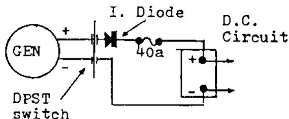
WIRING DIAGRAM FOR PRIMITIVE "CONTROL BOX" ON 110 VOLT WIND GENERATOR (PRIMARILY AN ANTI-MOTOR DEVICE, AND PROTECTION AGAINST LIGHTNING)
