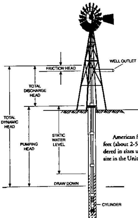
American farm windmills are available in sizes ranging from 6 feet to 16 feet (about 2-5 meters) in diameter. Australia's Southern Cross can be ordered in sizes up 25 feet (about 8 meters) in diameter. The most common size in the United States is the 8-foot mill.
