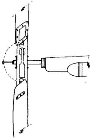
View showing how vane pullout spring is attached, and its position with the tail vane in operating position or when folded.
