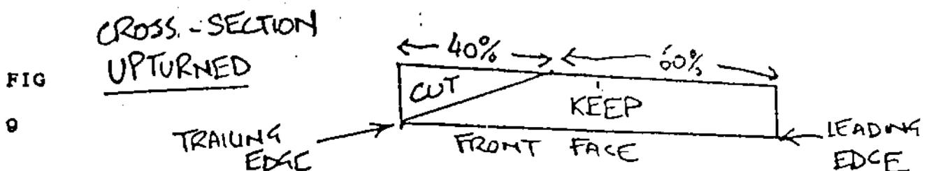
Finally you need to round off the sharp corners on the back of the blade, to produce a smoothly curved airfoil shape. I do this by eye really. Draw a line on the back face about 25% of the width back from the leading edge, and leave this line untouched, or you will lose your thickness. Figure 10 shows the general idea:
