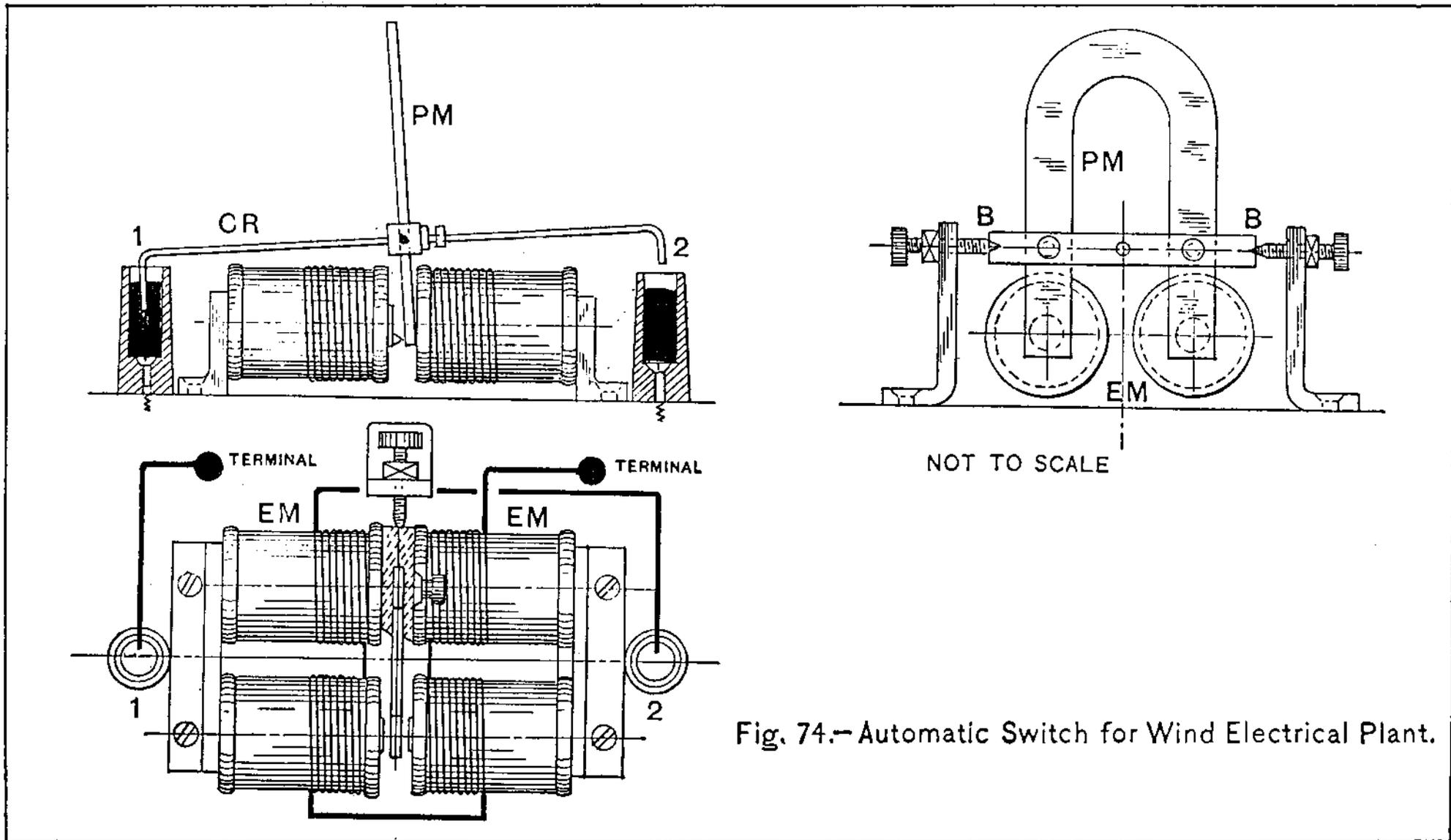
Fig. 74.—Automatic Switch for Wind Electrical Plant.
