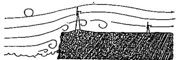
Severe turbulence may be created by the sea cliff in this example. As above, a higher tower will be required near the cliff while a shorter tower will be safe if placed at a great enough distance from the cliff.
