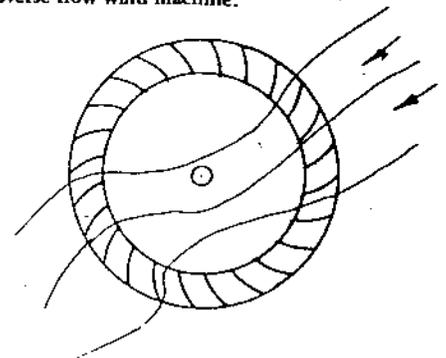
6b Transverse flow machine with flexible guide vanes which eliminate drag, and allow high rotation speeds.
