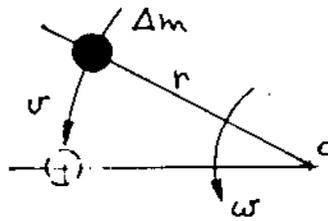
b Linear velocity  $v$  of particle,  $\Delta m$  rotating with angular velocity,  $\omega$ , about an axis through instantaneous centre of rotation,  $O$ .
