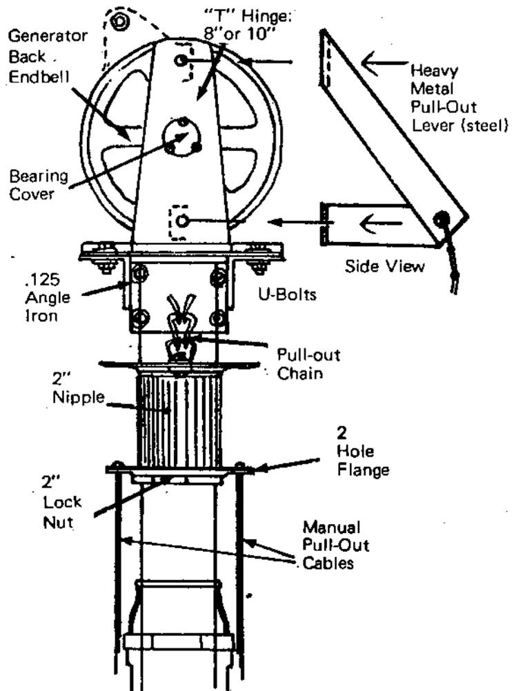
**Fig. 5 REAR VIEW OF GENERATOR AND PULL-OUT SYSTEM**
