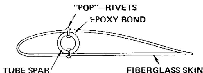
A few foam ribs may be bonded inside the fiberglass, but in any case, the fiberglass skin will be four to eight laminations thick, and must be strong enough to avoid flexing in strong winds.
