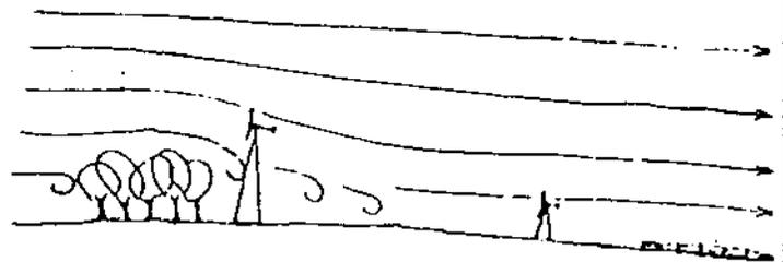
The grove of trees in this example will produce turbulence. A higher tower close to the trees places the wind generator above the turbulence. A shorter tower is safe if placed far enough away from the trees.
