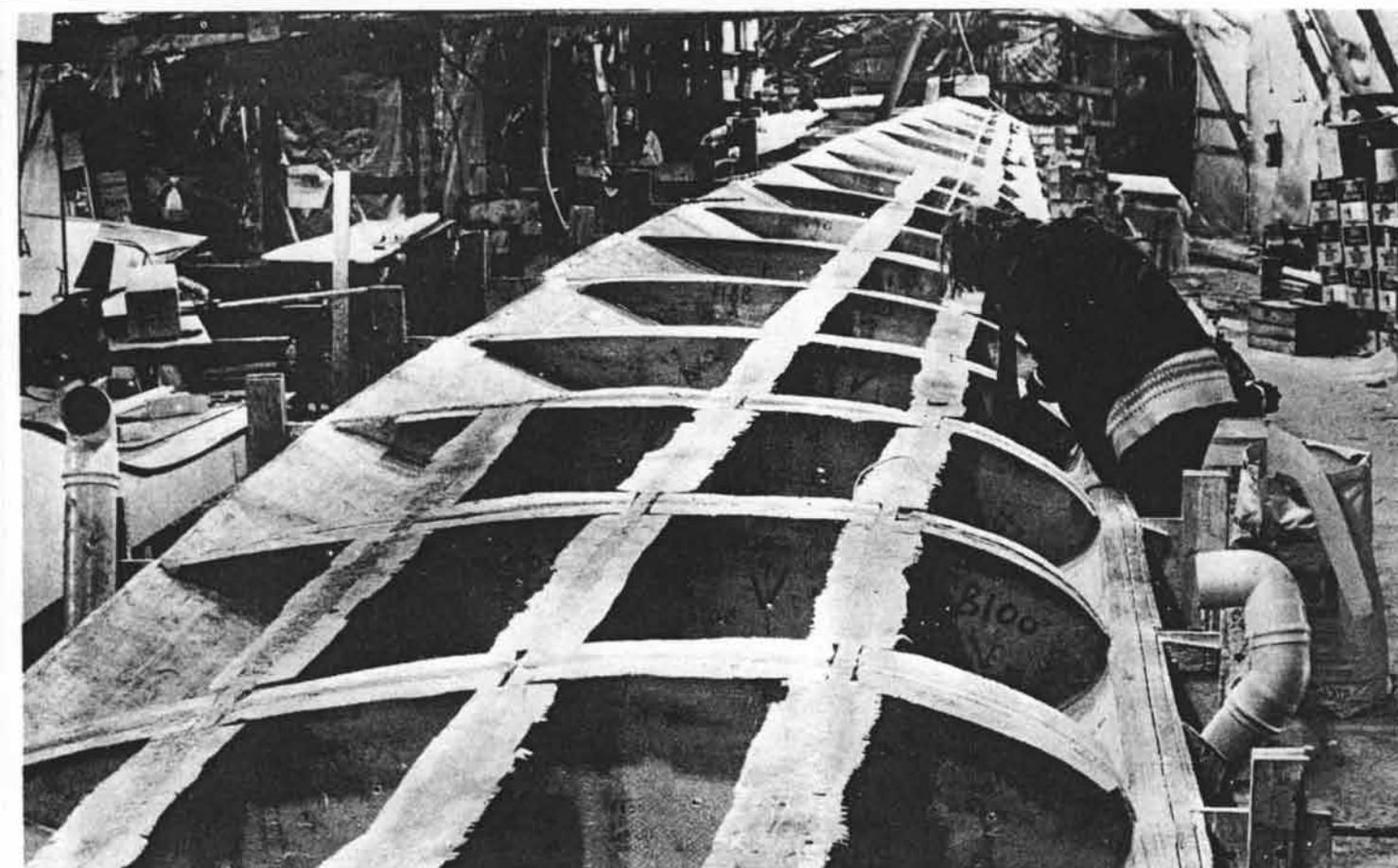
**Wing-Sections with sawn-out "Flamingo"- Polystyrol blocks.**
