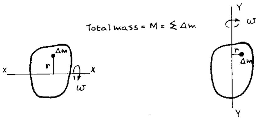
a. Moment of inertia about X-X axis,  $I_{xx}$ , is greater than moment of inertia of same body about Y-Y axis,  $I_{yy}$ .
