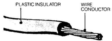
Metric cables are specified by the copper area (in square millimetres), the number of strands of wire and the number of conductors or cores in each sheath. The voltage drop is the same regardless of voltage, assuming that amps, distance and cross sectional areas are the same. If the wattage remains the same for different voltages, the amps can be calculated by dividing watts by volts.
