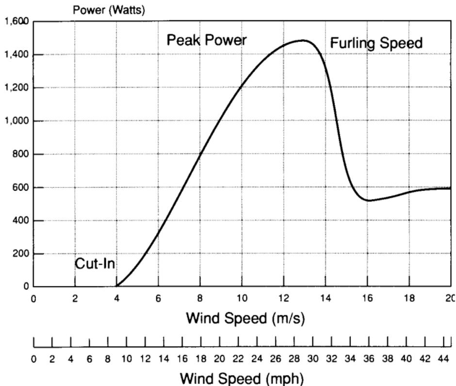
*Figure 4-2. Nomenclature for power curve of the Bergey 1500, a small wind machine 3 meters (10 feet) in diameter. (Bergey Windpower)*
