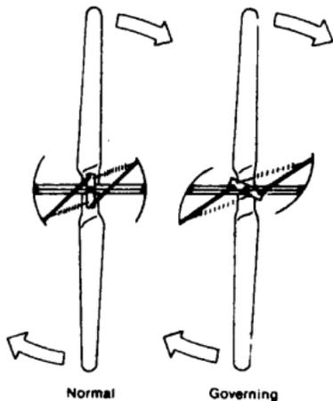
Slanted "Brake Shoes" cause air drag and slow rotor in high winds.
