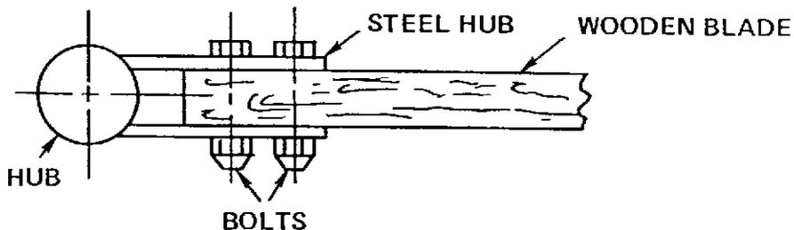
Notice in the sketch that the blade load ends up in two hub parts, which means that half of the load goes into each side of the blade. Thus 10,000 pounds is loaded at two different places along the attachment bolt - called double shear. Two 5/16 inch bolts could handle this load. In the case of wood blade attachment, lots of smaller bolts are recommended.
