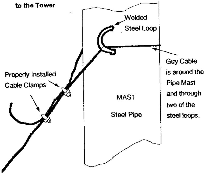
Above: the correct method of attaching the clamps to the guy cables. Note that the U-bolt side of the clamp is placed over the unused, free end of the guy cable.
