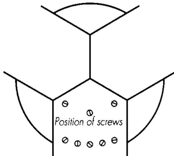
Each blade root must be cut to a point (Fig. 4.6) to fit snugly at the hub. Measure the exact centre of each blade root, and draw lines out to the edges, at an angle of  $60^\circ$  to each edge. Mark them front and back, then cut along the lines.
