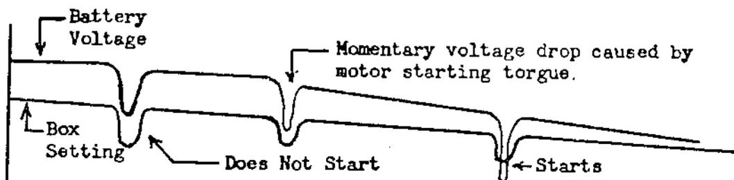
Sentry Box Voltage Setting:-Notice how the heavy current surges momentarily lower the box settings and prevent the engine starting on the majority of the power load cycles.
