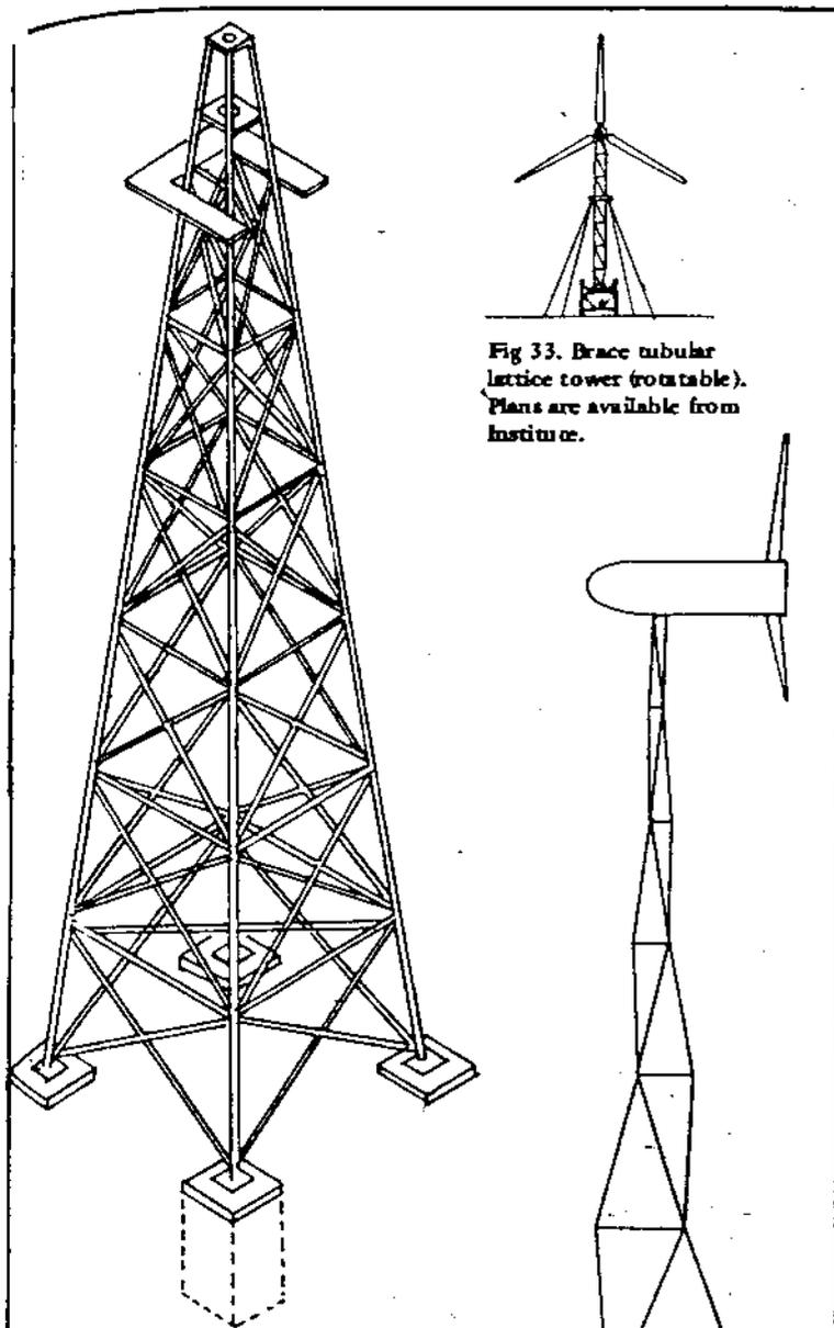
Fig 33. Brace tubular lattice tower (rotatable). Plans are available from Institute.
