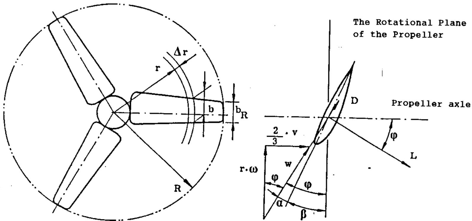
Figure 1. The Coordinates of the Propeller Blade
