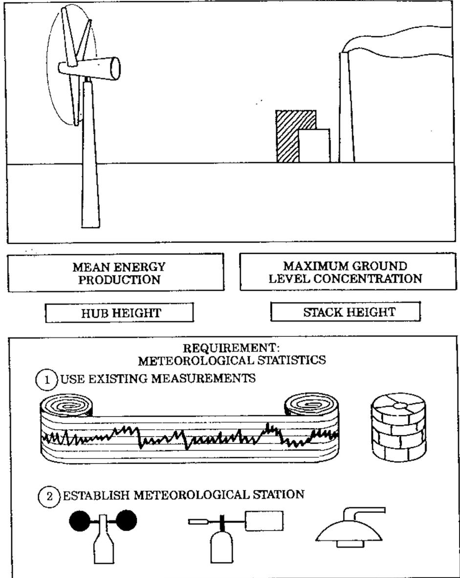
Figure 1. Meteorological statistics and two areas of application: Air pollution and wind energy.
