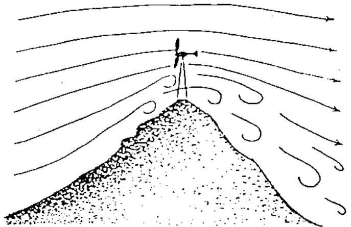
This drawing illustrates the proper location and height for a tower on this hill. It is fully exposed to the high-velocity winds and is above the region of harmful turbulence.
