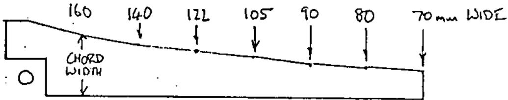
Turn the blade on edge, and work down to the line to an accuracy of plus/minus 1mm, and keep the cut face square to the "top" of the wood (see fig 4). Where there is more than 10mm of wood to remove, it may be easiest to cut through the waste across the grain with a saw and then chop out chunks with a chisel, along the grain. Or you can use a bandsaw if you have access.
