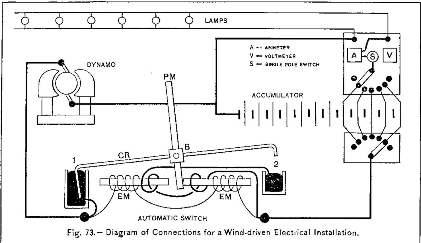
Fig. 73.— Diagram of Connections for a Wind-driven Electrical Installation.
