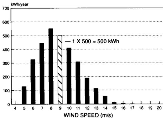
*Figure 4-3. Power curve method of calculating annual energy output. At 9 m/s the Bergey 1500 will produce 1 kilowatt. At a site with a 5.5 m/s (12.3 mph) average wind speed and a Rayleigh frequency distribution, winds occur at this speed 500 hours per year. Winds in the 9 m/s bin contribute 500 kilowatt-hours of the wind machine's total annual generation.*
