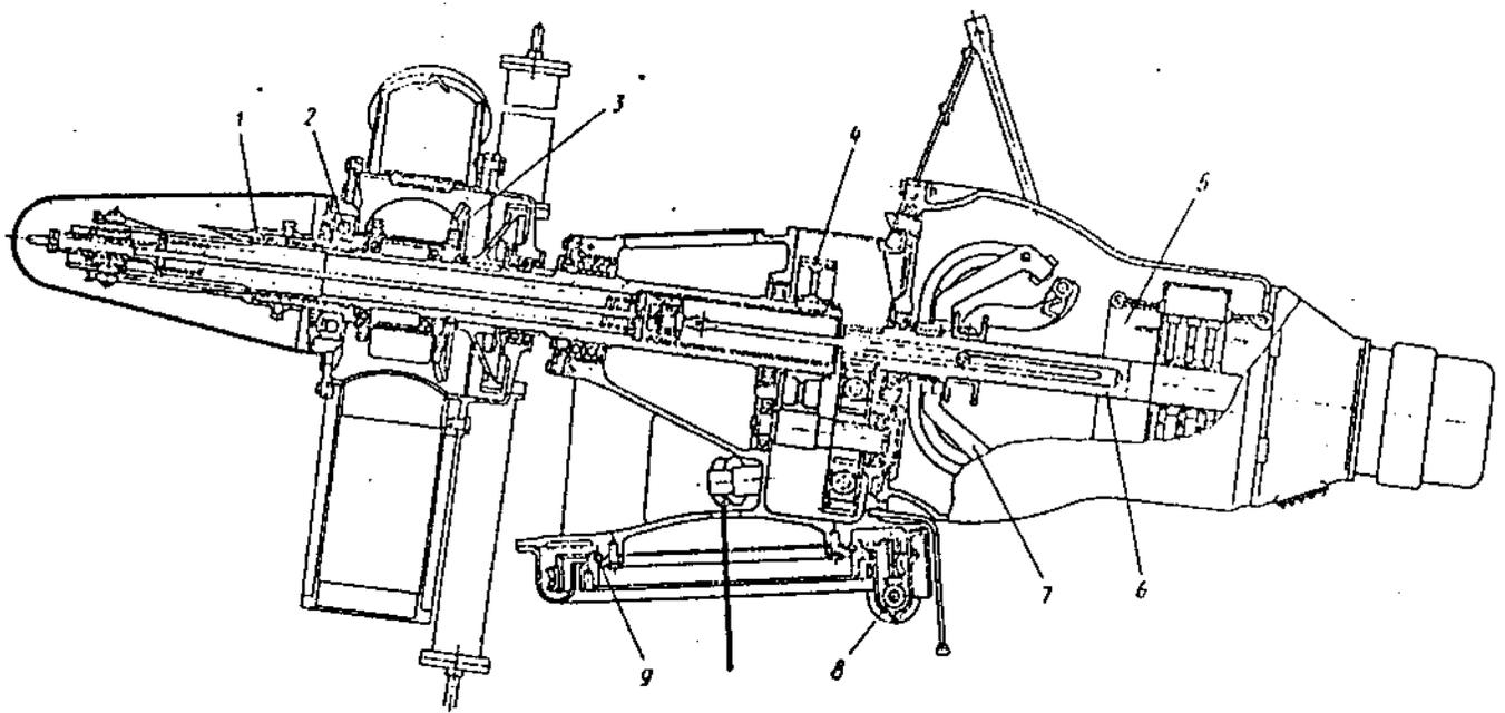
Fig. 81. Head of the "Sokol" machine: 1. main shaft; 2. bearing; 3. gear; 4. reduction gear; 5. generator; 6. generator shaft; 7. centrifugal regulator; 8. orientation mechanism; 9. support bearing.
