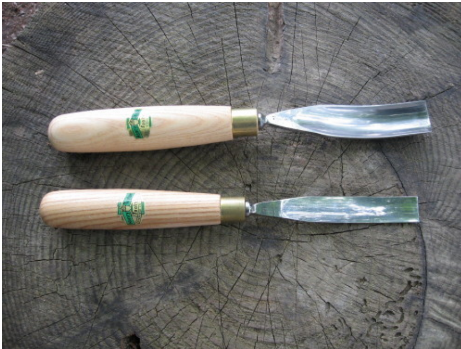
Gouges Deeply curved and flat gouges by Henry Taylor Tools, Ltd., Sheffield, England.
