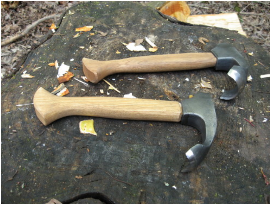
Woodcraft adzes Larger bowl adze at top, smaller cup adze at bottom.
