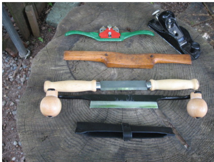
Finishing tools Top to bottom: metal and wood spokeshaves, Frosts splitting knife, drawknife, and block plane at top right.
