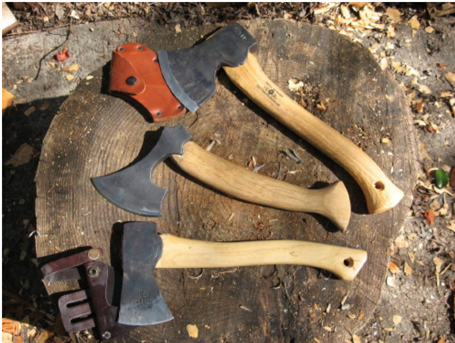
Three smaller carving axes Gransfors Bruks Swedish carving axe (at top), Woodcraft Scandinavian carving axe (middle), and Wetterlings small hunter (bottom). All three are fine axes for carving, but the upswept blade and heavier head make the GB better for heavy work.
